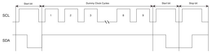
Figure 4-2. Bus Timing (SCL: Serial Clock, SDA: Serial Data I/O®)
