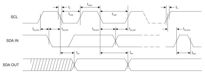
Figure 4-3. Write Cycle Timing (SCL: Serial Clock, SDA: Serial Data I/O)
